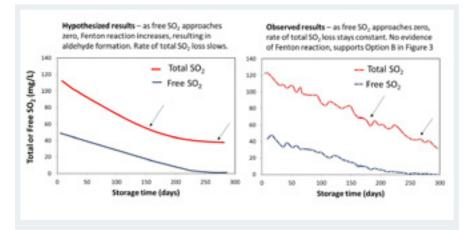
**FIGURE 5** (left) Hypothetical total and free  $SO_2$  versus storage time if new  $SO_2$  binders are generated during oxidation; (right) Observed total and free  $SO_2$  over time for a representative Chardonnay wine. Data replotted from (Sacks et al. 2020).
