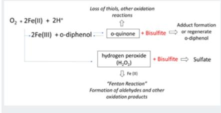
FIGURE 2 Overview of "iron-phenolic" oxidation pathway. Bisulfite limits to appearance of oxidative changes to wine (browning, aldehyde formation thiol loss) by reacting with initial oxidation products (hydrogen peroxide, quinones).
