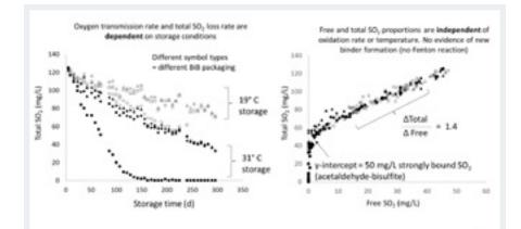
**FIGURE 4** (left) Total SO<sub>2</sub> vs. storage time in Chardonnay wine stored in different BiB packages at room and elevated temperature; (right) Total SO<sub>2</sub> vs. free SO<sub>2</sub> plots for BiB wine storage treatments. Plots adapted from (Sacks et al. 2020).
